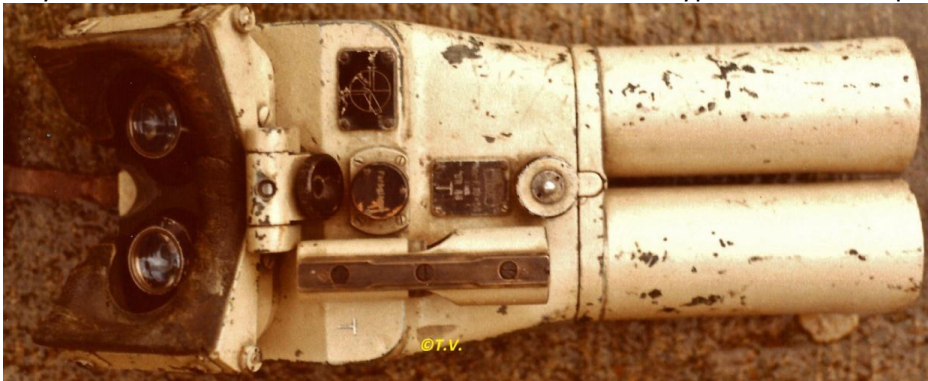
Pict 36 a, b; 12x60 blc Kriegsmarine model; reticle illuminating lamp; ©Anna Vacani
