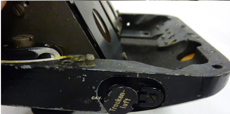
Pict 28 a, b, c; 12x60 rln trocken luft- air drying system ©Anna Vacani
