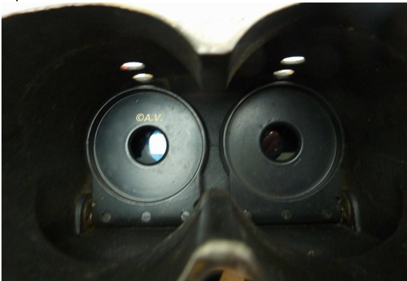
Pict 21; 12x60 bic model; Prod Nr 269084; closed diaphragm inside of the hood; ©Anna Vacani
