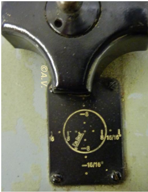
Pict 47; the plate on our 12 x 60 blc Kriegsmarine model; © Anna Vacani It helps to calculate a distance from an object. The remaining binoculars described in this article have a common reticule.
