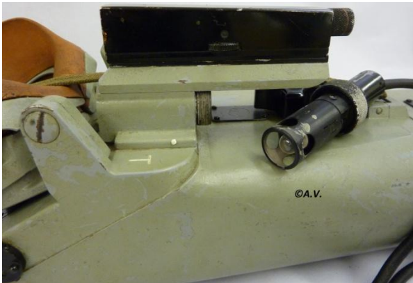
Pict 36 a, b; 12x60 blc Kriegsmarine model; reticle illuminating lamp; ©Anna Vacani
