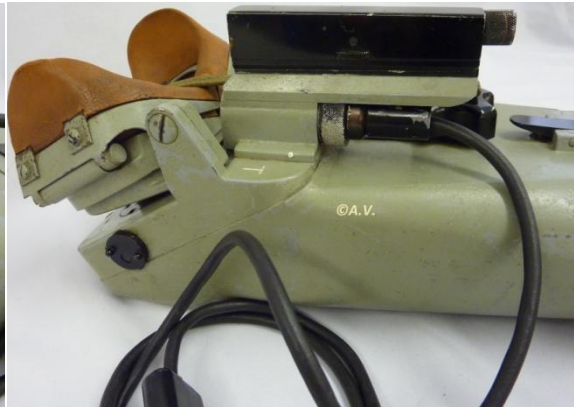
Pict 36 a, b; 12x60 blc Kriegsmarine model; reticle illuminating lamp; ©Anna Vacani
