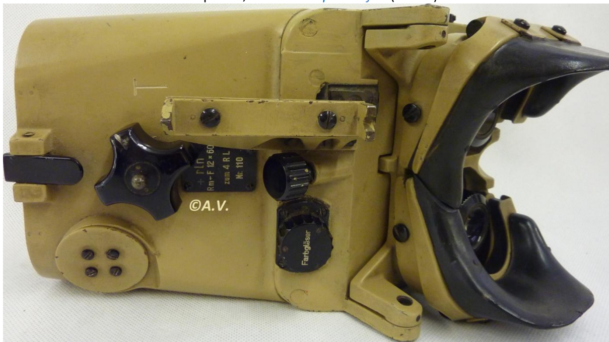
Pict 8; 12x60 Carl Zeiss Jena, marked “rln” model with symbol “+”; Prod Nr 259427; ©Anna Vacani The pictured model was intended to use in the low temperature environments. It has “+” symbol indicated that with this kind of grease the binocular can be used in temperature up to -40C.
