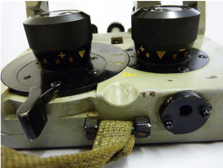
Pict 31 & 32 a; 12x60 blc Kriegsmarine model; Interpupillary distance mechanism; ©Anna Vacani
