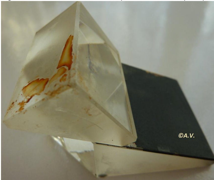
Pict 42 a; 12x60 blc Kriegsmarine model; two prisms – bottom one is silvered; ©Anna Vacani
