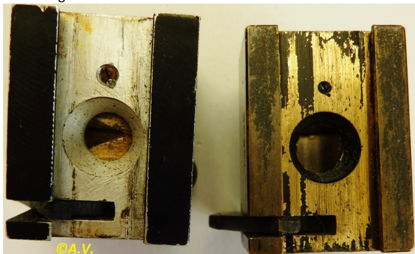
Pict 39; reticle illuminating lamps housings; left party closed, right opened; ©Anna Vacani
