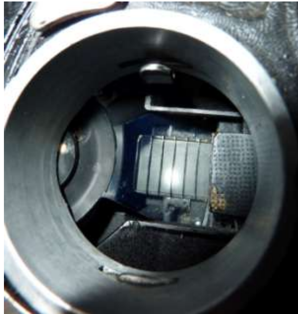
Reflex mirror shutter in our Arriflex camera
