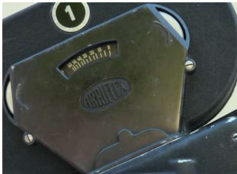
Picture of the magazine (200 ft-60 meters) fitted on our camera with the film counter
