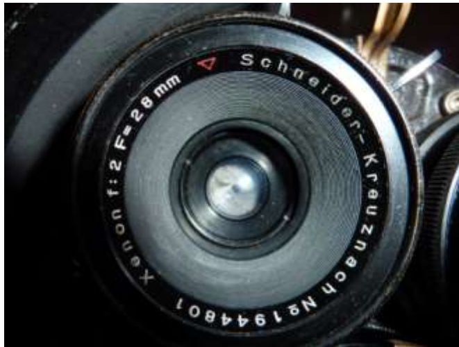
And Schneider- Kreuznacht Xenon f: 2, 3; F5 cm objective; focus 0 – 20 meters and infinitive:
