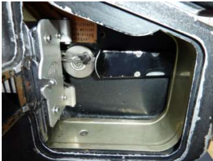
The film chamber in our camera
