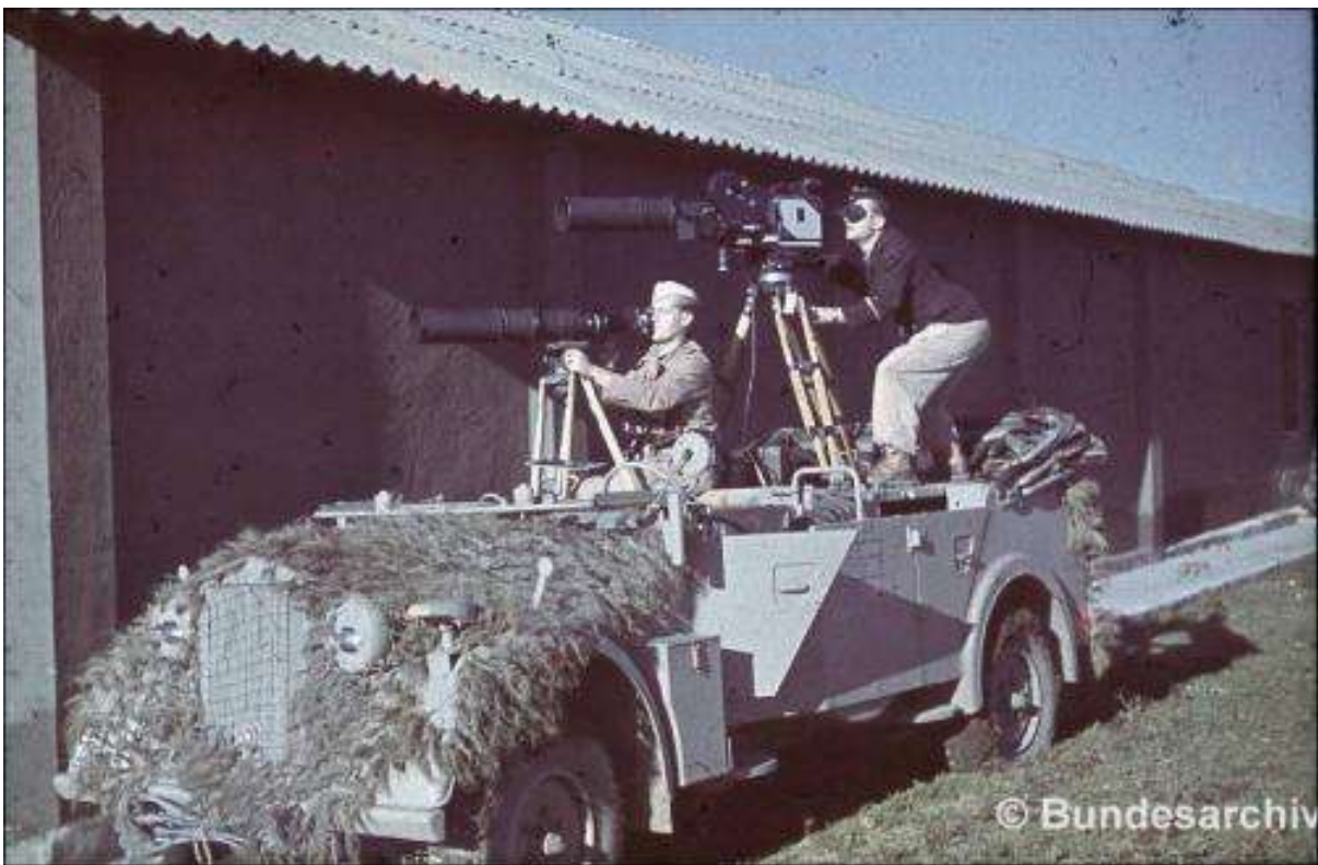
Two cameras Arriflex and Askania placed on the car using one tripod - 1943 Picture source: BArch, N 1603 Bild-255 Image/Horst Grund 4
