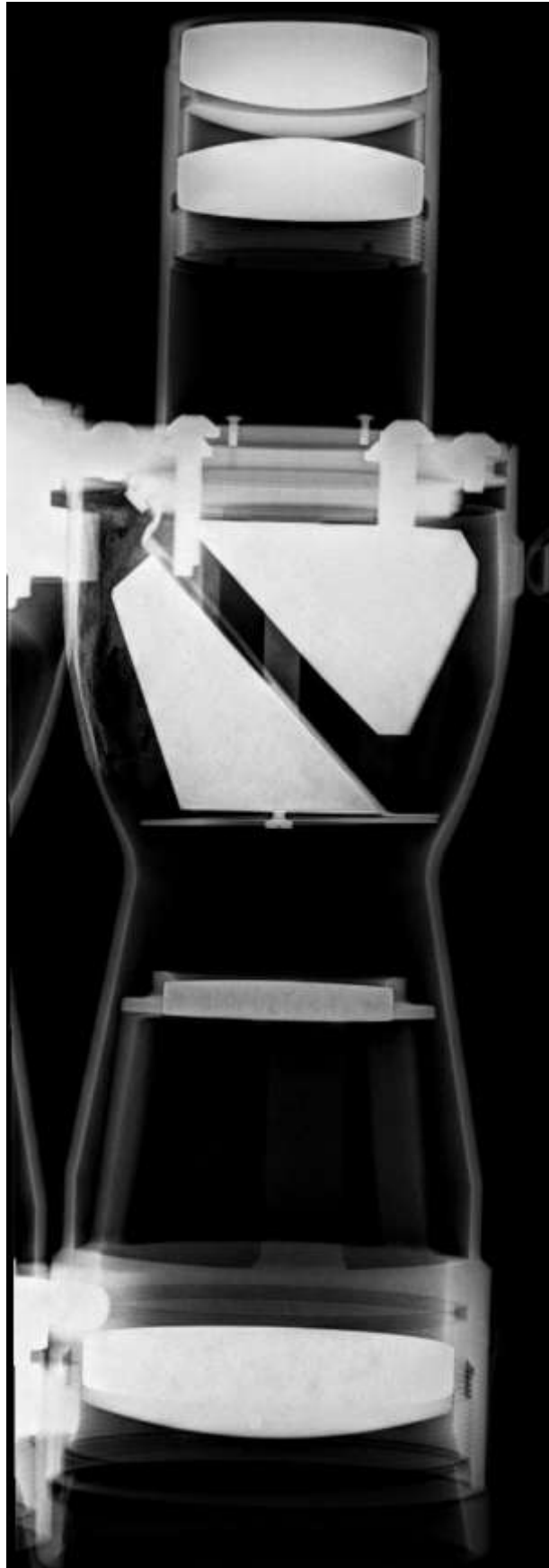
Pict.6. x-ray of the glasses inside of the Avimo prototype
