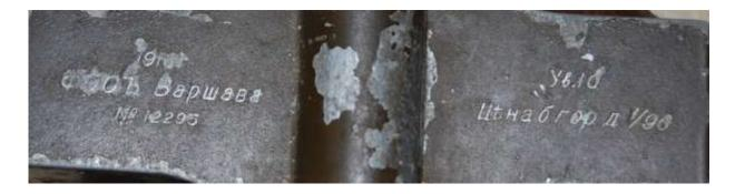
The description on the scissor binocular: left side – 1910y, FOS Warsaw No12295; right side – magnification 10, graduations of the reticule plate 1/90
