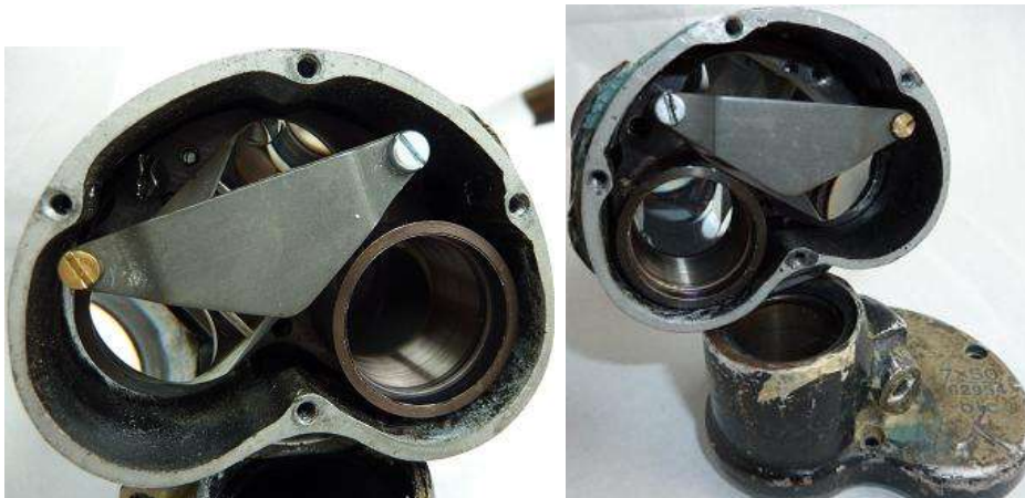
Pict 89; 7 x 50 U-boat, with the optic visible, production No 63954 taken apart from our collection; Copyrights of the picture Anna Vacani
