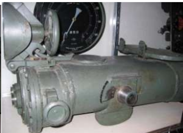
Pict 36, 37; 20x120 type 97 from Richard Lane collection; Pictures taken by R. Lane; Copyrights R. Lane Richard Lane says: "The Type 97 binocular prisms are actually larger than a standard Japanese WWII 20x120 (several millimetres on each face)."
