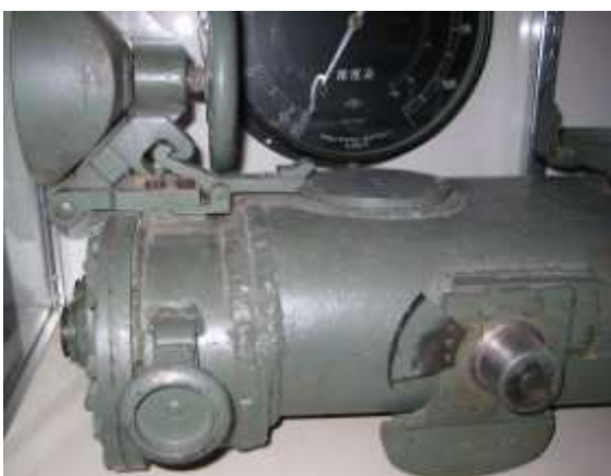
Pict 36, 37; 20x120 type 97 from Richard Lane collection; Pictures taken by R. Lane; Copyrights R. Lane Richard Lane says: "The Type 97 binocular prisms are actually larger than a standard Japanese WWII 20x120 (several millimetres on each face)."
