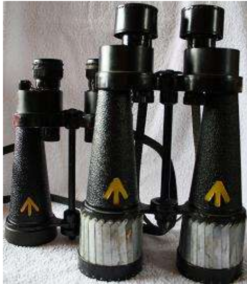
Pict 57; Barr & Stroud CF41 7x50 – with and without desiccator connections, from James Stewart collection, kindly sent for this article; Copyrights pictures James Stewart
