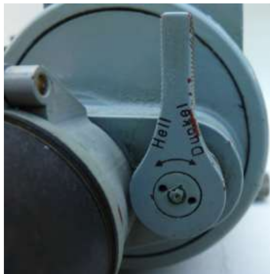
The external lever of the illumination mechanism
