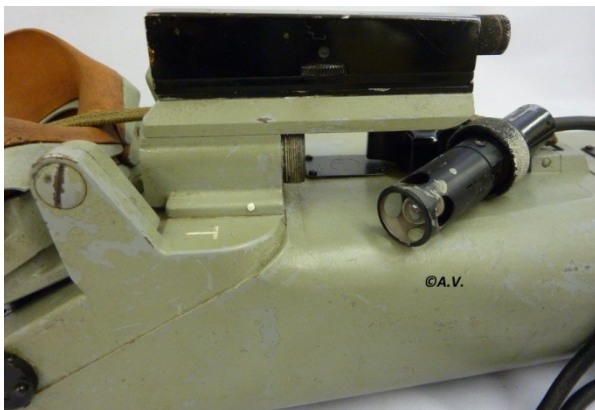
Pict 43 a, b; 12x60 blc Kriegsmarine model; reticle illuminating lamp; ©Anna Vacani
