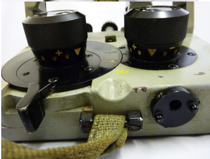
Pict 38 a & b; 12x60 b/c Kriegsmarine model; Interpupillary distance mechanism; ©Anna Vacani
