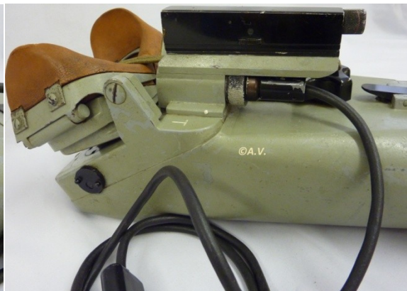
Pict 43 a, b; 12x60 blc Kriegsmarine model; reticle illuminating lamp; ©Anna Vacani
