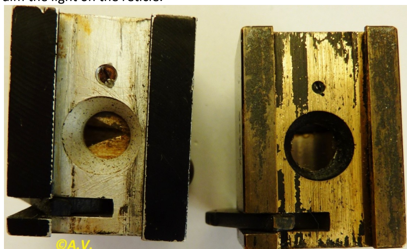
Pict 46 a; reticle illuminating lamps housings; left party closed, right opened; ©Anna Vacani
