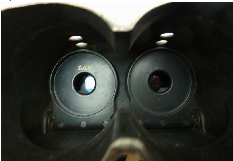
Pict 21; 12x60 bld model; Prod Nr 269084; closed diaphragm inside of the hood; ©Anna Vacani
