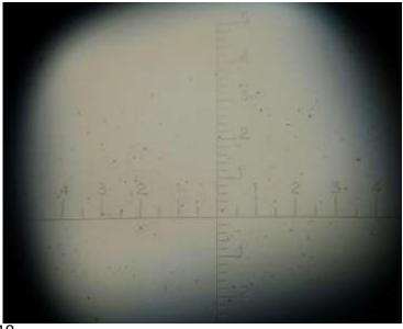
The reticule in the right eye piece tube of the H.Kolberg binocular-1925
