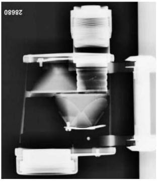
The x-ray picture of the H.Kolberg binocular (production 1930)
