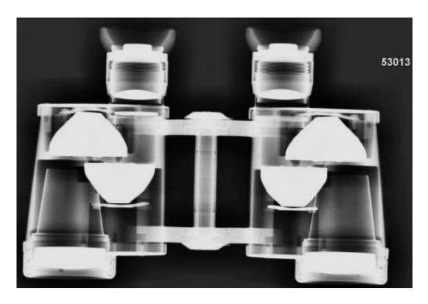
The x-ray picture of the OPW binocular (production No 53013)
