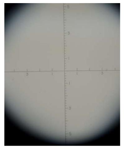
The reticule in the right eye piece tube of the H.Kolberg binocular-1930
