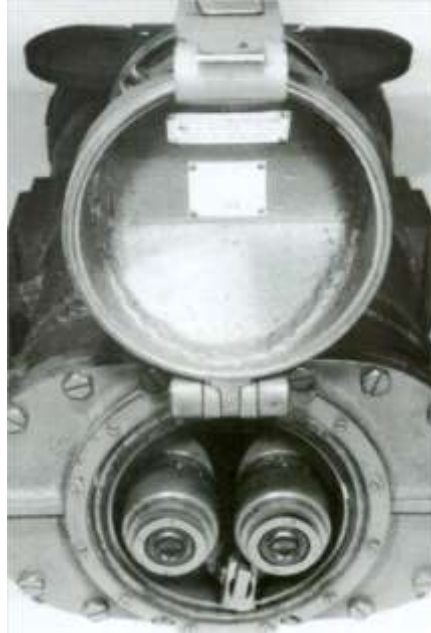
A CLOSER VIEW OF TO REAR WATERTIGHT HATCH WICH IS CONTROLLED BY A LOCKING WHEEL. THE EYEPIECES CAN BE ADJUSTED FOR EYE SEPARATION. ON THE INSIDE SURFACE OF THIS HATCH IS THE IDIDENTIFICATION PLATE. IT SHOWS A PRODUCTION DATE OF OCTCBER 1944 WITH THE SERIAL NUMBER 311. ALSO PRESENT IS THE NIKKO LOGO USED BY NIPPON KOGAKU; BOTH BEFORE, DURING AND AFTER THE WAR. R. LINE
