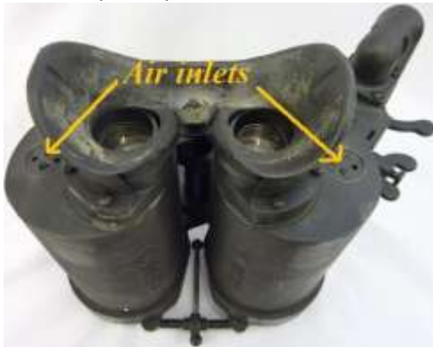
Pict 53; Bausch & Lomb MK 91 Mod 1; the air inlets; copyrights pictures
