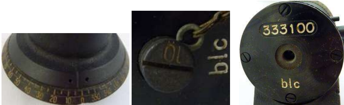
Pict 76; The base with oil compartment and the bolt
