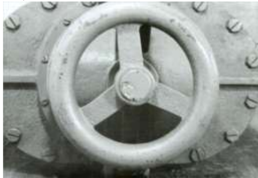
A CLOSER VIEW OF TO REAR WATERTIGHT HATCH WICH IS CONTROLLED BY A LOCKING WHEEL. THE EYEPIECES CAN BE ADJUSTED FOR EYE SEPARATION. ON THE INSIDE SURFACE OF THIS HATCH IS THE IDIDENTIFICATION PLATE. IT SHOWS A PRODUCTION DATE OF OCTCBER 1944 WITH THE SERIAL NUMBER 311. ALSO PRESENT IS THE NIKKO LOGO USED BY NIPPON KOGAKU; BOTH BEFORE, DURING AND AFTER THE WAR. R. LINE
